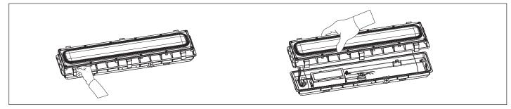
1. Unfasten the latches and separate the led module and the power housing.
