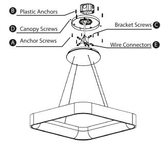
Step 3. Remove Plastic Pin, drill 4 (8mm) holes on the ceiling according the Mounting Bracket. Insert the expansion bolts in the holes.
