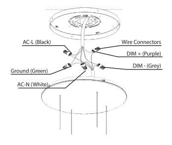
Step 6. Adjust the fixture safety cable and Aircraft cable length, use Screw to adjust the Mounting Bracket and Mounting Canopy. Keep the fixture level as possible line up the slots on the bottom fixture mount bracket with the canopy screw. Rotate until until both bracket are in place tighten canopy screws to secure it in place. Lossen all the cables
