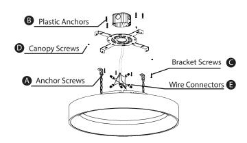
Step 3. Remove plastic pin, drill 4 (8mm) holes on the ceiling according the mounting bracket.
