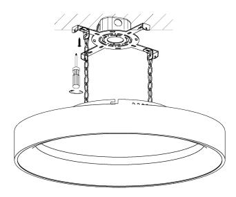
Step 6. Keep the fixture level as possible line up the slots on the bottom fixture mount bracket with the canopy screw. Rotate until until both bracket are in place tighten canopy screws to secure it in place.
