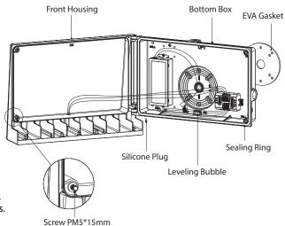
Note: To ensure waterproof seal, apply weatherproof silicone sealant between the mounting surface and mounting box, as well as around the sides of housing. This is especially important with an uneven wall surface. Silocne all plugs and unused conduit entries.
