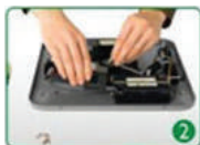
Replacing Power Supply
