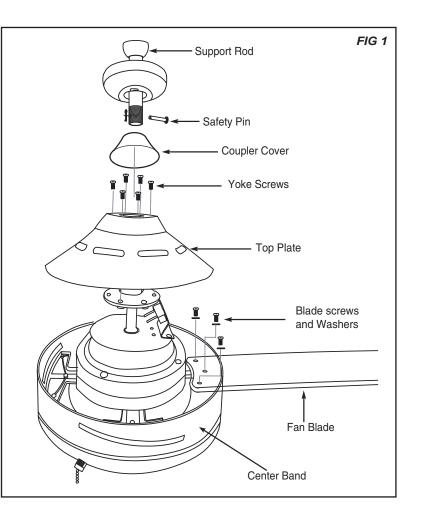
Back off (loosen) the set screws (2) in the support rod coupler until the inside of the channel is clear of the screw tip. Remove and save the safety pin and washer on the end of the support rod assembly. Slide the ceiling canopy onto the support rod, followed by the support rod coupler cover (see *figure 1*). Feed the electrical wires from the fan housing through the support rod.
