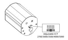
5 Insert driver into mounting hole, leaving fixture cable exposed.
