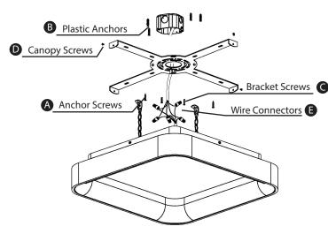
Step 3. Remove plastic pin, drill 4 pcs or 6 pcs diameter 6mm holes on the ceiling according the mounting mracket. (Note: the fixture dia is bigger than  $2' \times 2'$  (including  $2' \times 2'$ , need 6pcs holes, 4 for bracket screw, 2 for safety bracket screw). Insert the plastic anchors into the holes. (Use 2 pcs M4 x 25mm screws to secure mounting bracket with J-Box, refer to picture shown below. See Fig. 2
