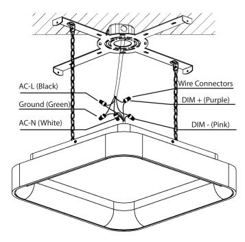
Step 7. Ensure that the fixture is secure. Turn on the power at breaker box or main fuse box to see the fixture is in working order.
