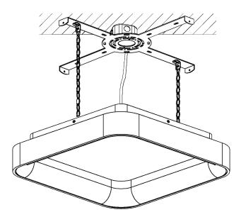
Step 5. Use wire connectors L, N, B, DIM+, DIM - wires. After making the connections place the wires with connectors into the J-Box.
