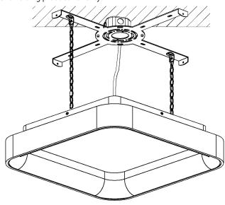
Step 6. Keep the fixture level as possible line up the slot hole while pushing upwards. Place canopy screws into slot holes using a screwdriver to secure the fixture.
