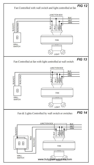
*Figure 13* illustrates the wiring used to control fan with the pull chain on the electrical switch housing plus an optional light fixture with a wall switch.
