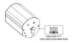
5 Insert driver into mounting hole, leaving fixture cable exposed.
