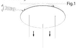
Step 3. Remove Plastic Pin, drill 4 (8mm) holes on the ceiling according the Mounting Bracket. Insert the expansion bolts in the holes.
