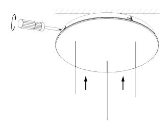
Step 7. Ensure that the fixture is secure. Turn on the power at breaker box or main fuse box. The fixture should illuminate if wired properly.
