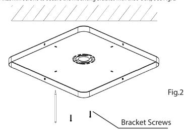
Step 4. Use 4 pcs M4x25 Self-Tapping Screw to secure the Mounting Bracket on to the ceiling.
