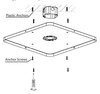
Step 6. Keep the fixture level as possible line up the slots on the bottom fixture mount bracket with the canopy screw. Rotate until until both bracket are in place tighten canopy screws to secure it in place.
