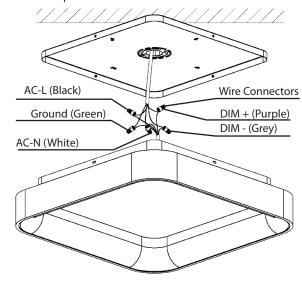
Step 7. Ensure that the fixture is secure. Turn on the power at breaker box or main fuse box. The fixture should illuminate if wired properly.
