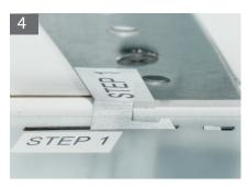
**Step 4:** Align the 2 longer hooks on the metal plate with the longer hole on the luminaire. "STEP 1" is marked on the luminaire. Insert the two longer hooks into the STEP 1 holes. Slightly move the luminaire forward and make sure the hooks are in firmly inserted.
