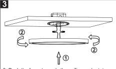
3. Push the lamp towards the ceiling and rotate the lamp to make the mounting plate and the lamp body fixed tightly.
