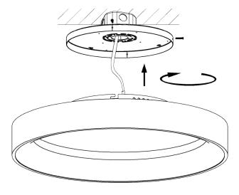
Step 7. Ensure that the fixture is secure. Turn on the power at breaker box or main fuse box. The fixture should illuminate if wired properly.
