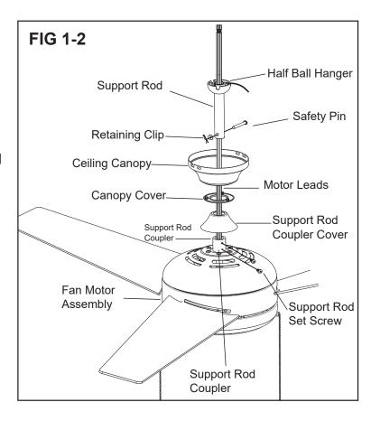
If you are using an extended support rod, (longer than the one supplied with your fan) remove the half ball from the support assembly and attach it to the extended support rod at this point. Make sure to retighten the set screw and insert the safety pin.
