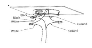
**Step 3.**Once all wiring is connect place wires in the junction box.
