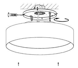
Step 5. Use wire connectors L, N, B, DIM+, DIM - wires. After making the connections place the wires with connectors into the J-Box.
