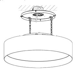
Step 6. Keep the fixture level as possible line up the slots on the bottom fixture mount bracket with the canopy screw. Rotate until until both bracket are in place tighten canopy screws to secure it in place
