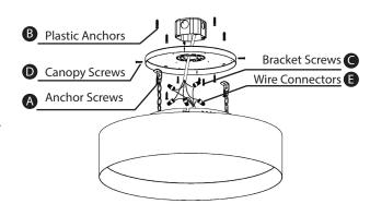
Step 3. Remove Plastic Pin, drill 6 (8mm) holes on the ceiling according the Mounting Bracket. (4 for the Bracket, 2 for safety Bracket Screws). Insert the expansion bolts in the holes. (Use 2 pcs M4x25mm screws to secure the Mounting Bracket with the J-Box), See Fig. 2
