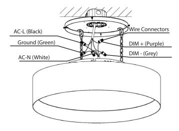
Step 7. Ensure that the fixture is secure. Turn on the power at breaker box or main fuse box. The fixture should illuminate if wired properly.
