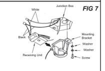
Attach the WHITE wire from the junction box to the WHITE wire from the receiving unit. Attach the BLACK wire from the junction box to the BLACK wire from the receiving unit (See **figure 7**).
