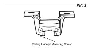
Install the mounting bracket onto the electrical junction box in the ceiling using two machine screws, two washers and two lock washers (see *figure 4*).
