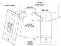
Step 3 Make the wire connections and secure them with wire nuts as shown in *figure 3*. Depending on where your power supply is located in reference to the wall control, *figure 3* will show you how to attach all of the necessary wiring. Since the wiring is quite different, make sure you know where your main power supply is located.
